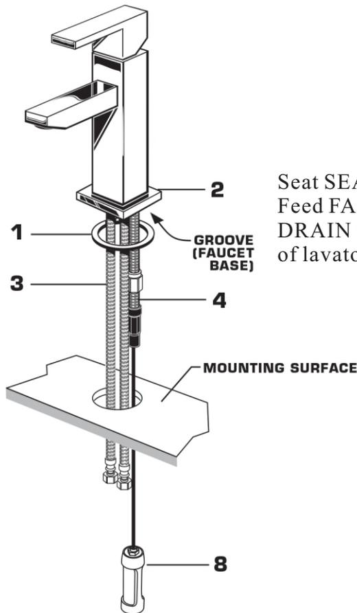
Seat SEAL [1] into under side of FAUCET BASE [2]. Feed FAUCET SUPPLIES [3], MOUNTING STUD [4] and DRAIN CABLE ASSEMBLY [8] through the mounting hole of lavatory or mounting surface.
