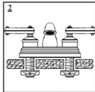
**2** Install faucet through holes in sink. From underneath sink put locknuts on faucet threaded shanks and properly tighten nuts by hand.
