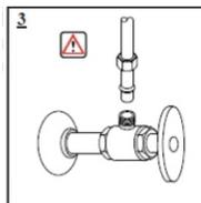
**3** Connect hot and cold faucet water supply lines to the water supply valves. Tighten connectors firmly being careful not to over tighten.
