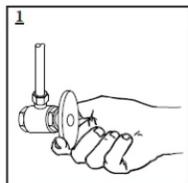
**1** Shut off water supply. Cover sink drain with cloth to avoid losing small parts. Remove old faucet. Clean sink surface in preparation for new faucet.
