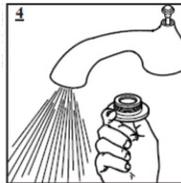
**4** After installation is complete, remove aerator. Turn water supply valves on beneath the sink and turn faucet on. Allow both hot and cold water to run at least one minute each. While water is running, check for leaks. Replace aerator.
