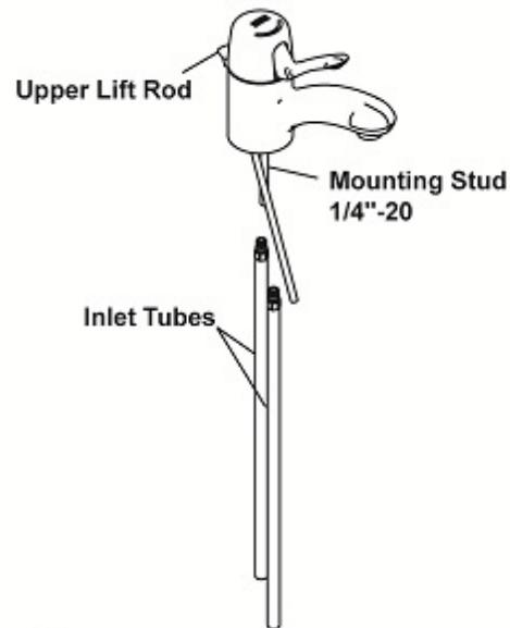
7. Place faucet and cover plate onto sink with inlet tubes through mounting hole. Use plumbers putty to seal faucet to sink. Place a ring of putty around hole openings of the sink base.
